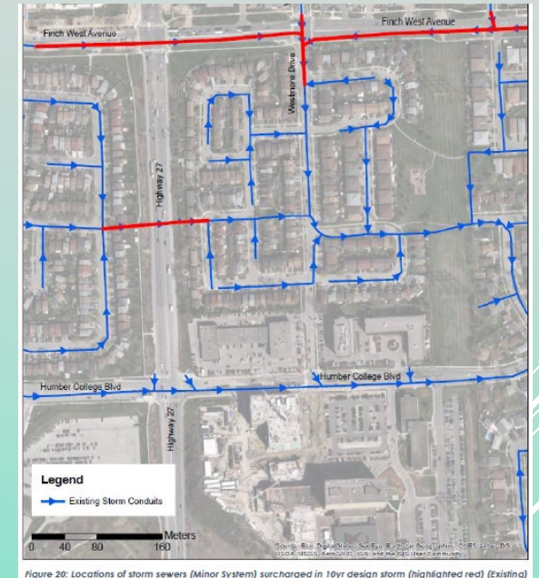
Figure 20: Locations of storm sewers (Minor System) surcharged in 10yr design storm (highlighted red) (Existing)
