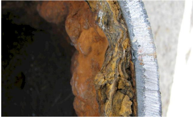
Internal Corrosion (Tuberculation) in Unlined Iron Pipe
