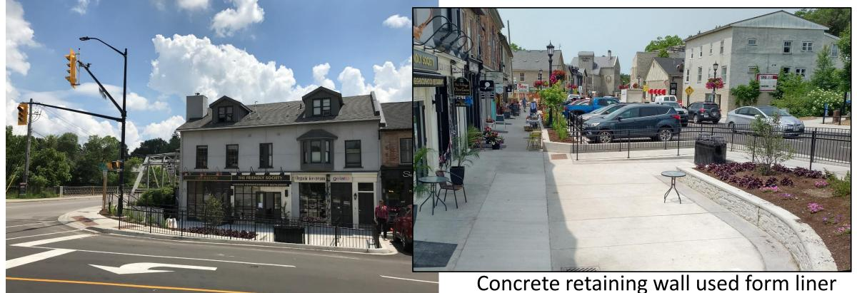
Concrete retaining wall used form liner for stone look to tie in with buildings
