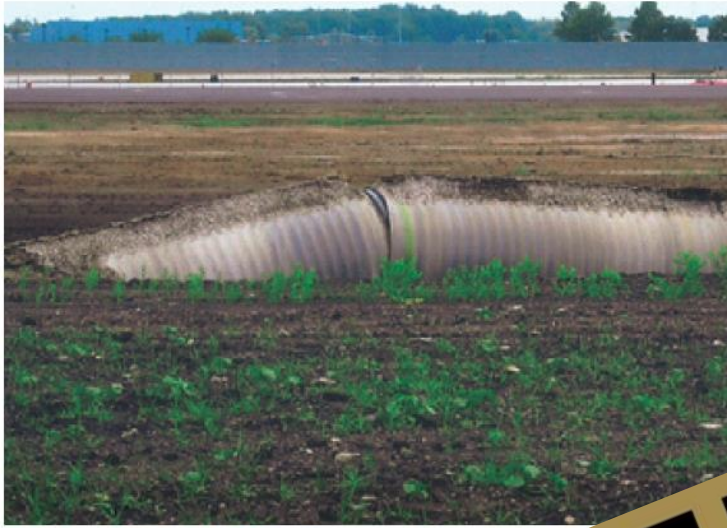
Columbus, Ohio Airport – polypropylene floating out of ground
